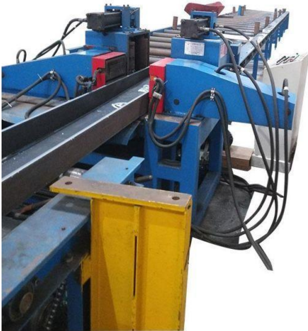
Assembling H beam in horizontal position
